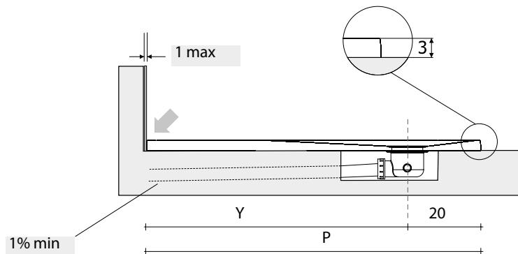
Montaggio in appoggio CX - Floor assembly CX - Bodenausführung CX
